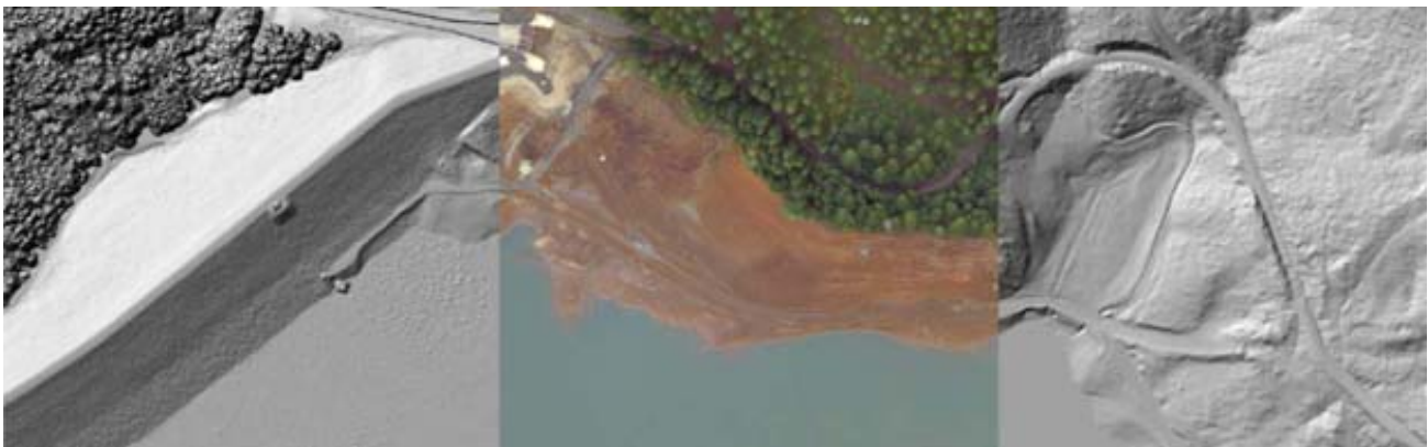
Three image types collected in the LiDAR survey: hillshade (left), air photo at 0.5 ft resolution (center), and bare earth image (right). Images by Watershed Sciences.
