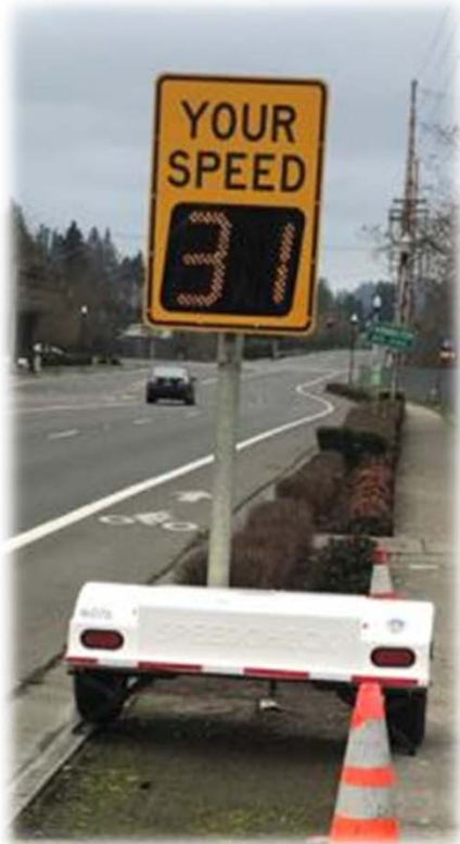
Speed display signs (radar trailer)
