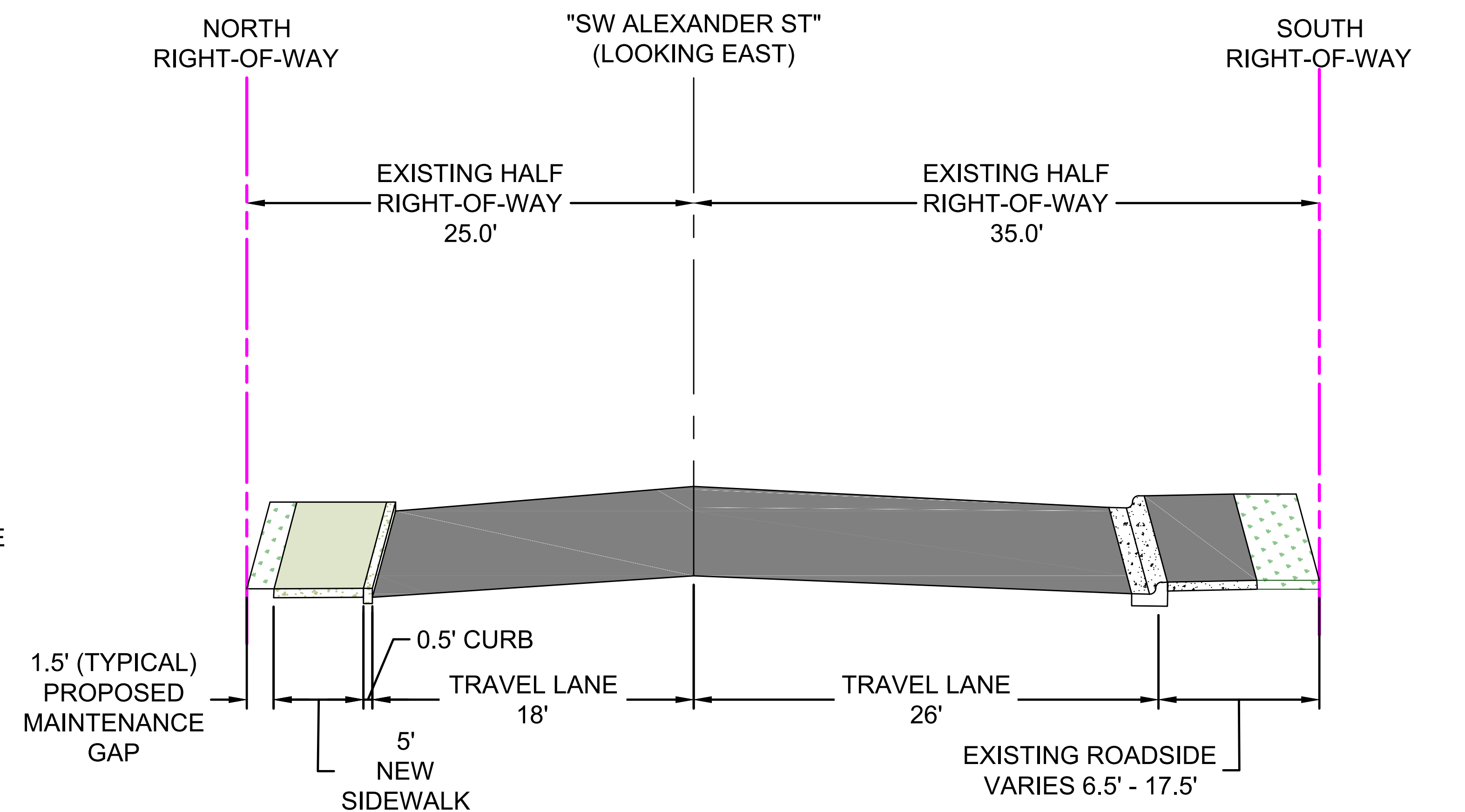
SW ALEXANDER STREET CURBTIGHT SIDEWALK - EAST INFILL
