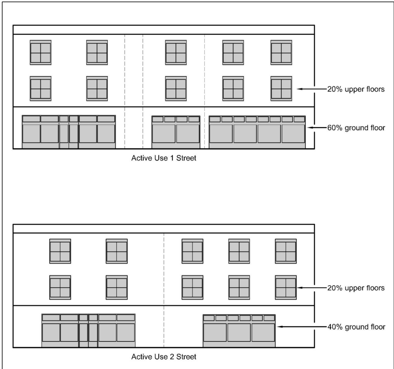
Figure 10 - Examples of Building Façade Transparency in the NCMU NB District (Elevation)
