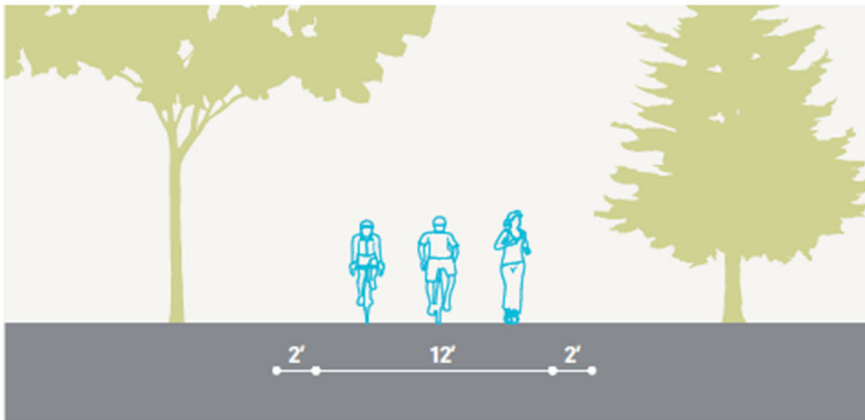
A 12-foot path with 2-foot shoulders is the typical design for a regional multiuse path.
