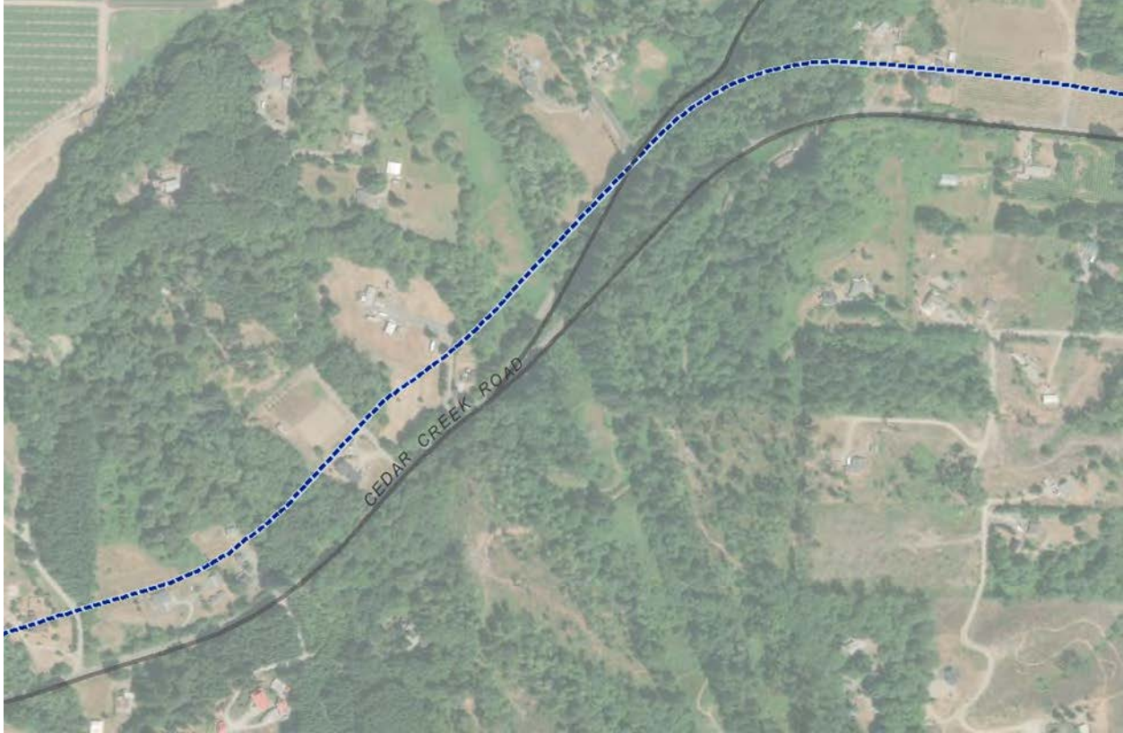
Figure 3. The Hayes Road/Cedar Creek Road 1996 ETR segment (in blue) was misaligned up to 250 feet.
