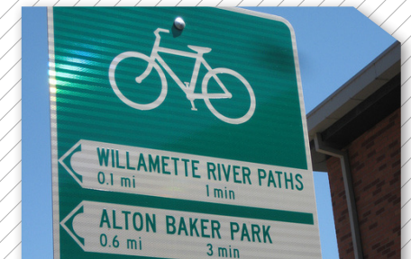
Wayfinding signage in Eugene, Oregon provides bicyclists with direction, distance and average ride time to key destinations
