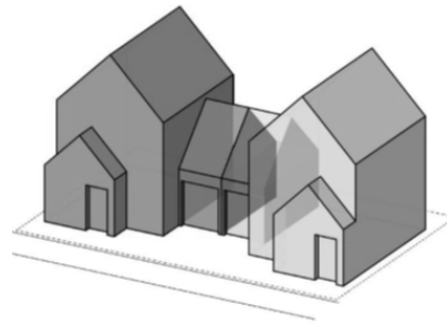
Attached by Garage Wall
