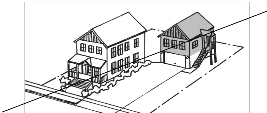
Section 106-6 Figure 3 – Detached (addition/conversion over detached garage)
